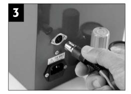
Plug the foot pedal into the back of the unit.
